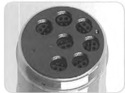
EXO2 sonde contains 6 universal sensor ports plus a central port for an anti-fouling wiper
