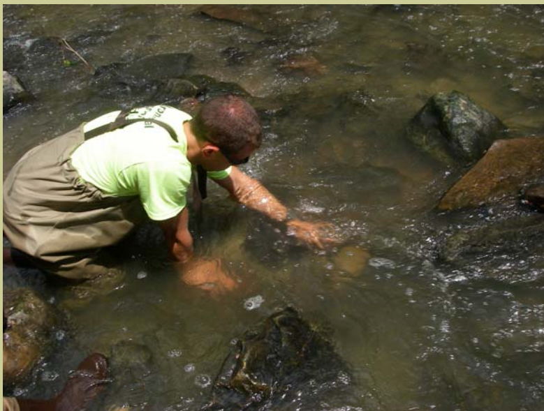
Installing a Hester-Dendy Artificial Substrate Sampler
