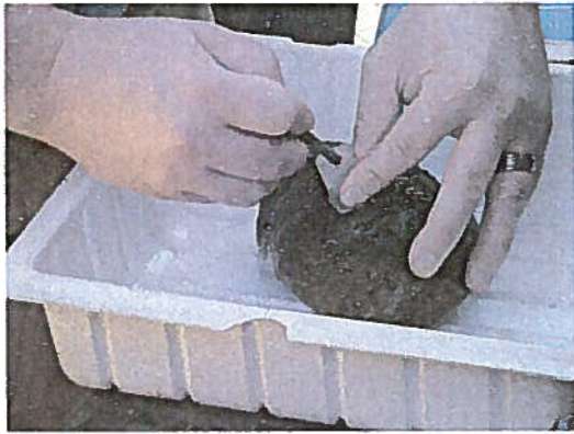
Figure 1. Scribing of circle inside syringe
