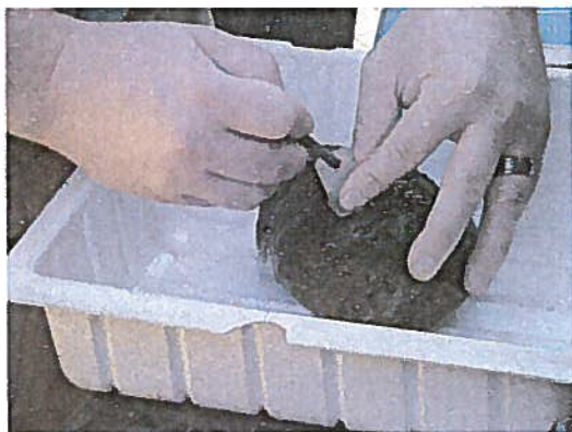
Figure 1. Scribing of circle inside syringe
