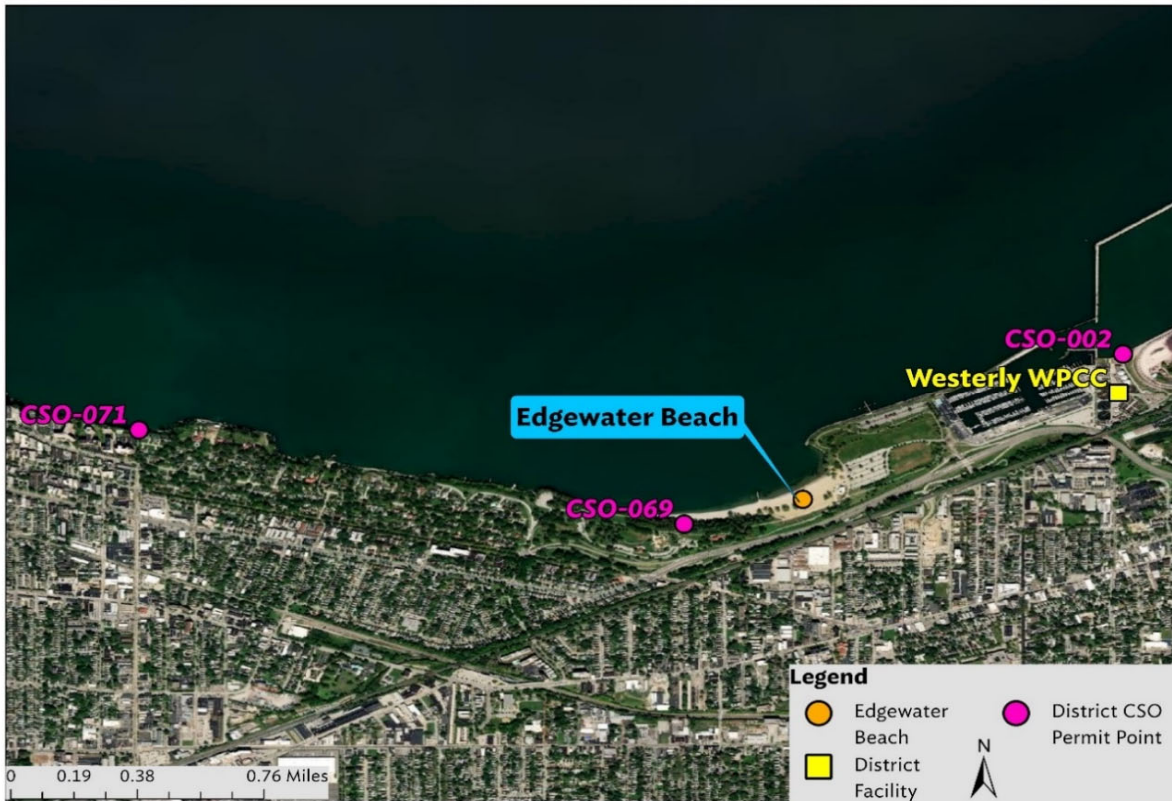
Figure 10. Proximity of CSO Outfalls to Edgewater Beach.
