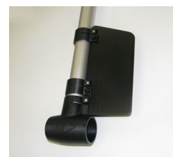
Flow probe prop housing with optional alignment fin.
