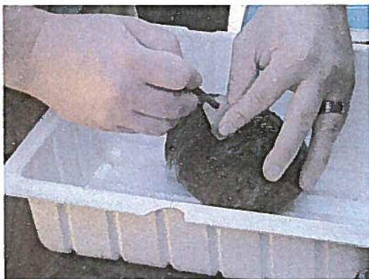
Figure 1. Scribing of circle inside syringe
