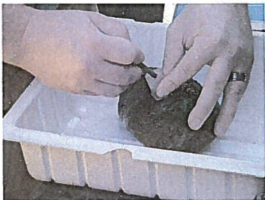
Figure 1. Scribing of circle inside syringe
