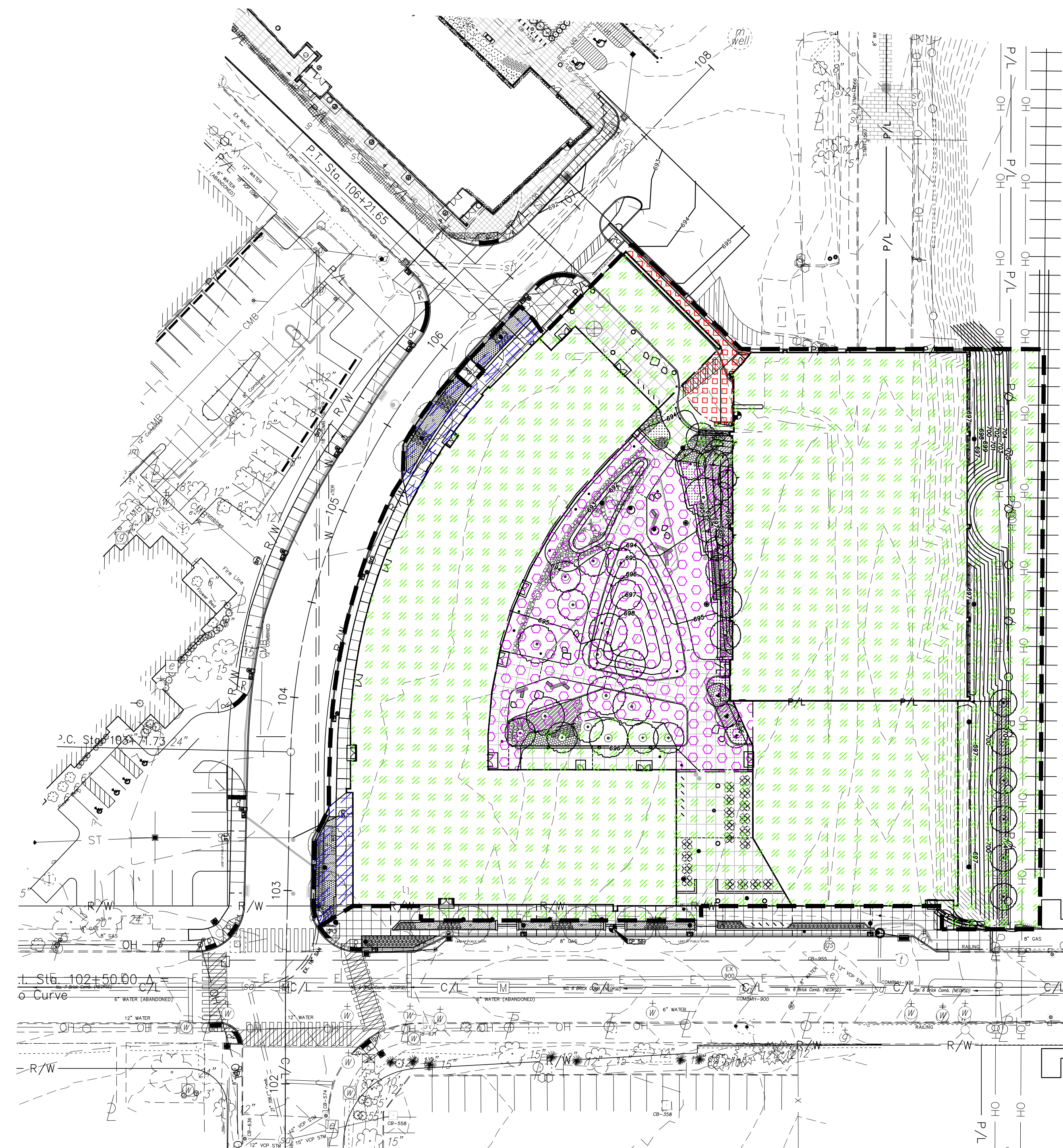
POST-BMP DETENTION AREAS
