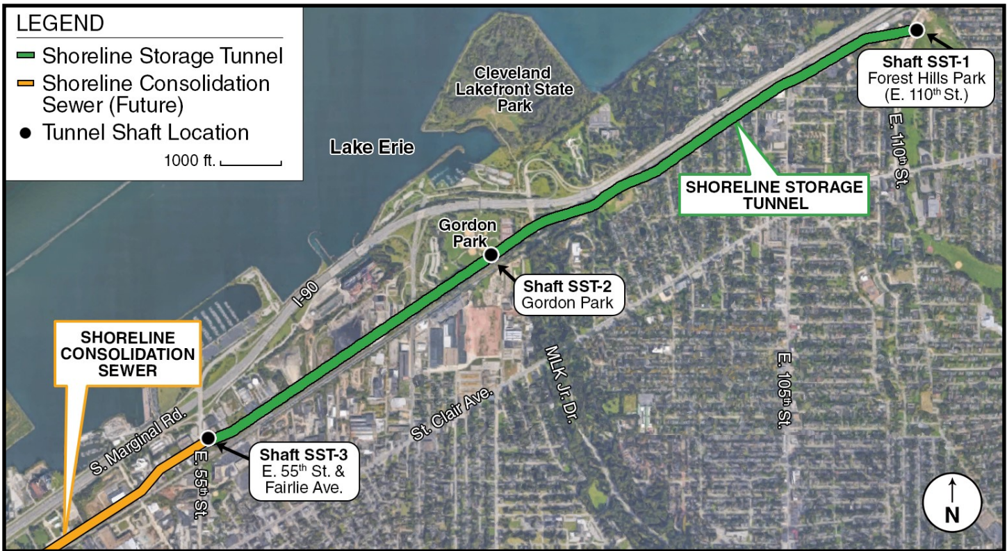
SST alignment map including three tunnel shafts
