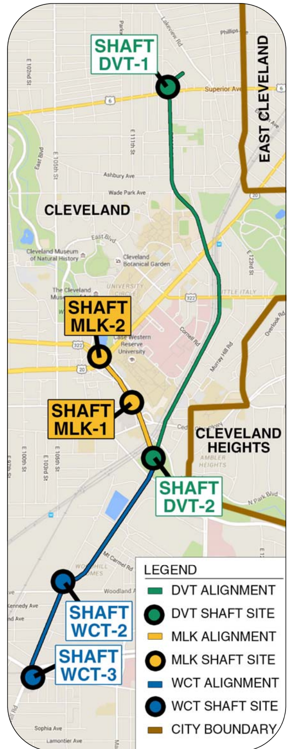
DVT alignment map, including all three tunnel segments (DVT, MLK & WCT) and six tunnel shafts
